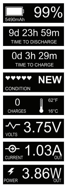
Shows the percent of charge remaining and the actual capacity remaining in mAh.
